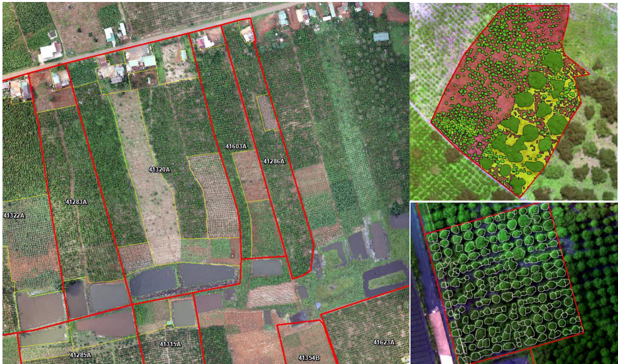
Figure 8. UAV mapped smallholder coffee farm boundaries with intra-plot sections (left); differentiation of exposed baresoil, weeds (upper right), shade trees and coffee plants; and mapped individual tree crowns (lower right)
