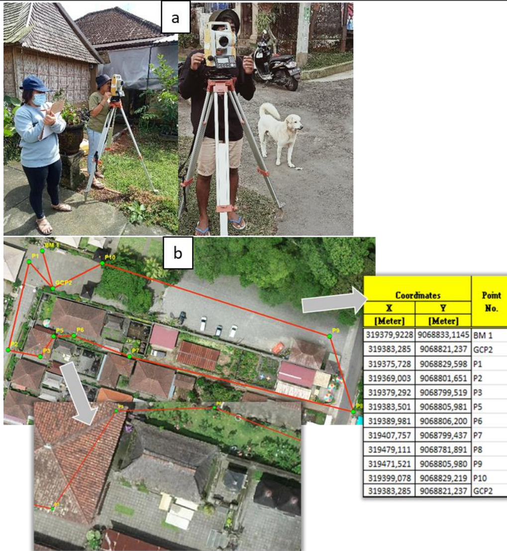
Figure 3. (a) Horizontal measurement documentation, (b) processing and plotting results
