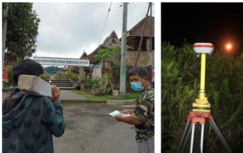
Figure 2. Installation of stakes or control points and GNSS observations using the GNSS (Author's documentation)
