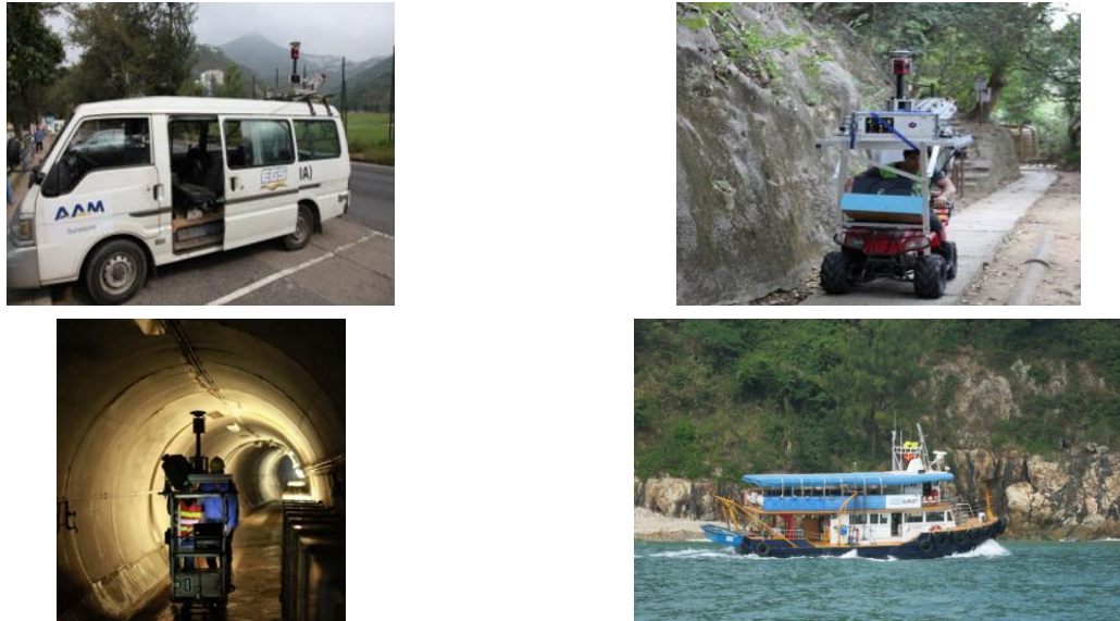
Figure 4: The MLS System Mounted on Different Mobile Platforms for Different Site Conditions
