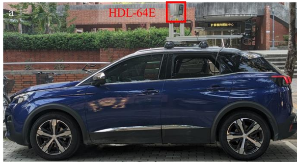
Figure 1. Mobile laser system a. PEUGEOT 3008 b. HDL-64E
