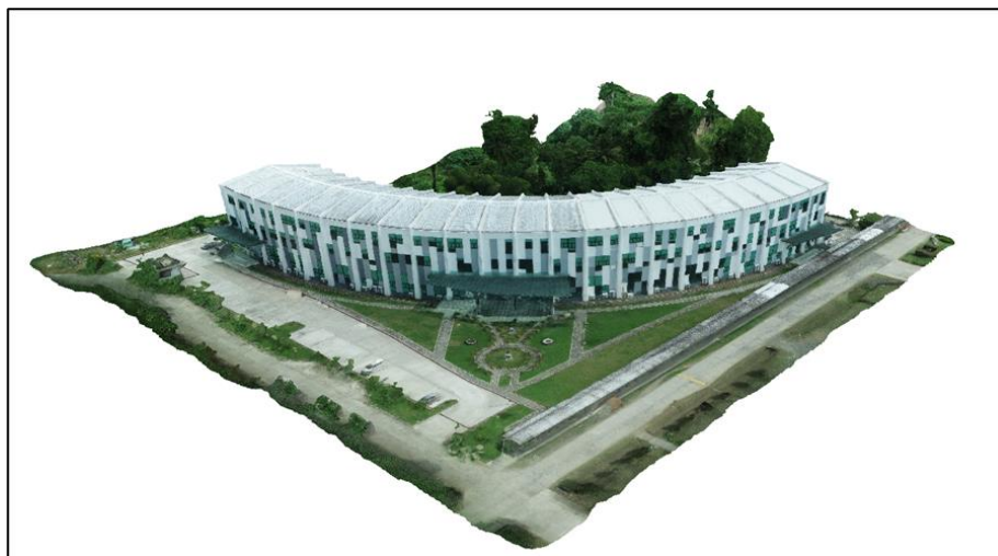
Figure 2. Digital Twin Model Generated using the First Set of Flight Plan Parameters
