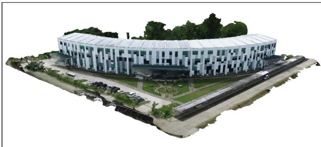
Figure 4. Digital Twin Model Generated using the Third Set of Flight Plan Parameters
