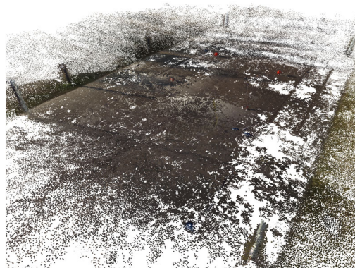
Figure 6. Processing result (the image acquisition interval was 0.5 m)
