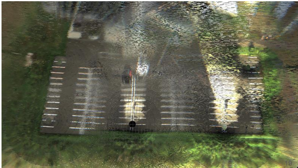
Figure 9 Five point measurement has combined and projected onto single 2d ground plane.
