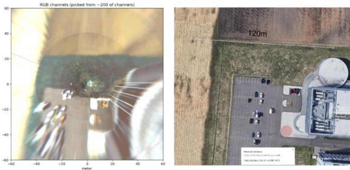
Figure 6. Left: RGB representation of spectral scan in 2D ground projection, Right: satellite imagery (Google maps) of the same position, Hokkaido University Campus.
