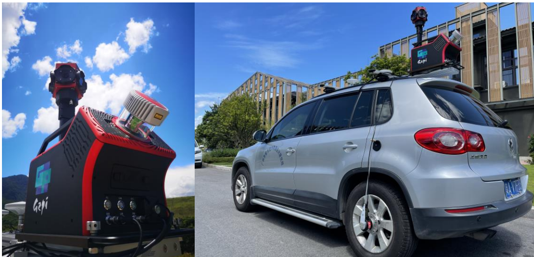
Figure 2 High-precision vehicle-mounted mobile measurement system
