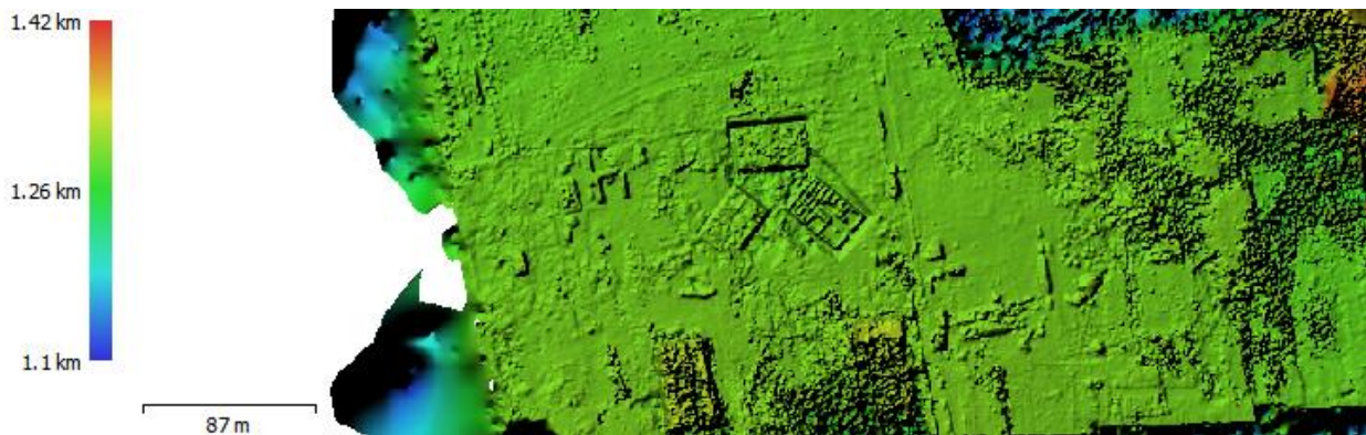
Figure 5. Sparse digital surface model (DSM) before densification obtained in the reprocessing process
