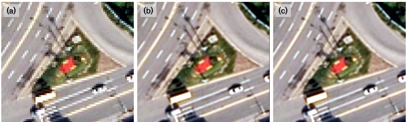
Figure 5. GCP chip GSD according to upsampling ratio. (a): ratio 1 (0.5m), (b): ratio 2 (0.25m), (c): ratio 3 (0.167m)
