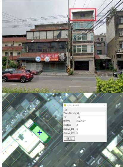
Fig.9 Data Adjustment on Newly Installed Building Story
