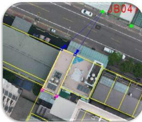
Fig.8 Building Polygon after Geometric Surveying
