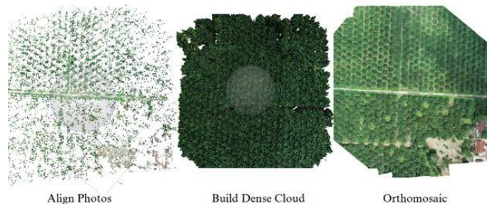
Figure 3. Processing of UAV orthophoto
