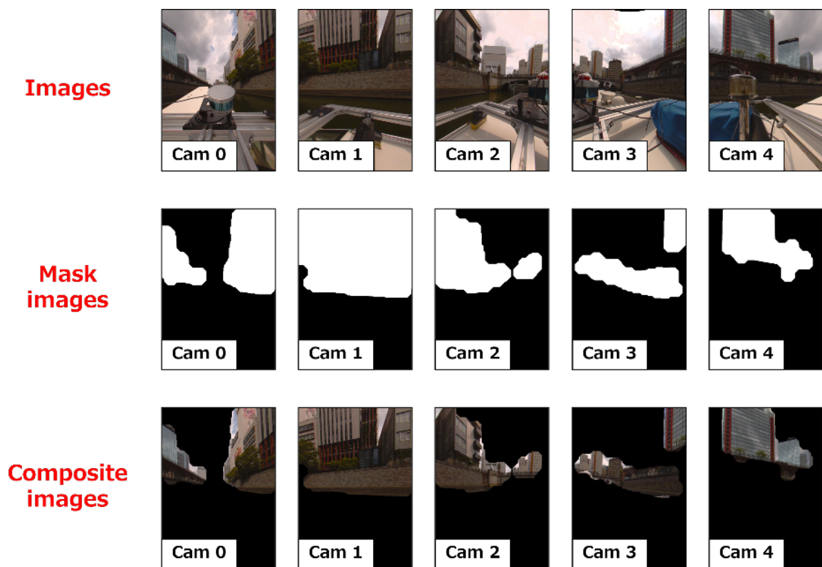
Figure 11: Example of mask processing results for omnidirectional camera images.
