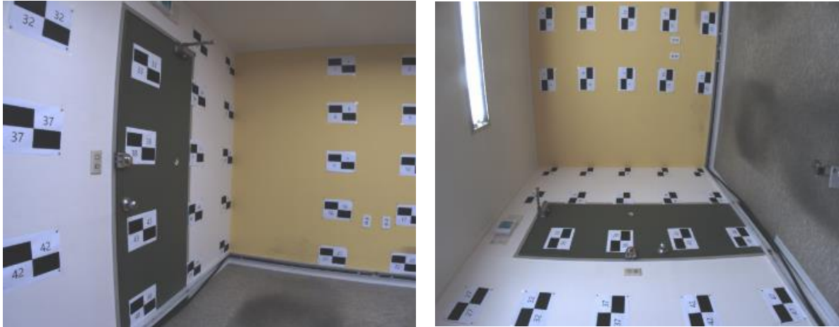
Figure 4. Camera calibration targets on test-bed wall (left: \kappa=0^\circ , right: \kappa=90^\circ )
