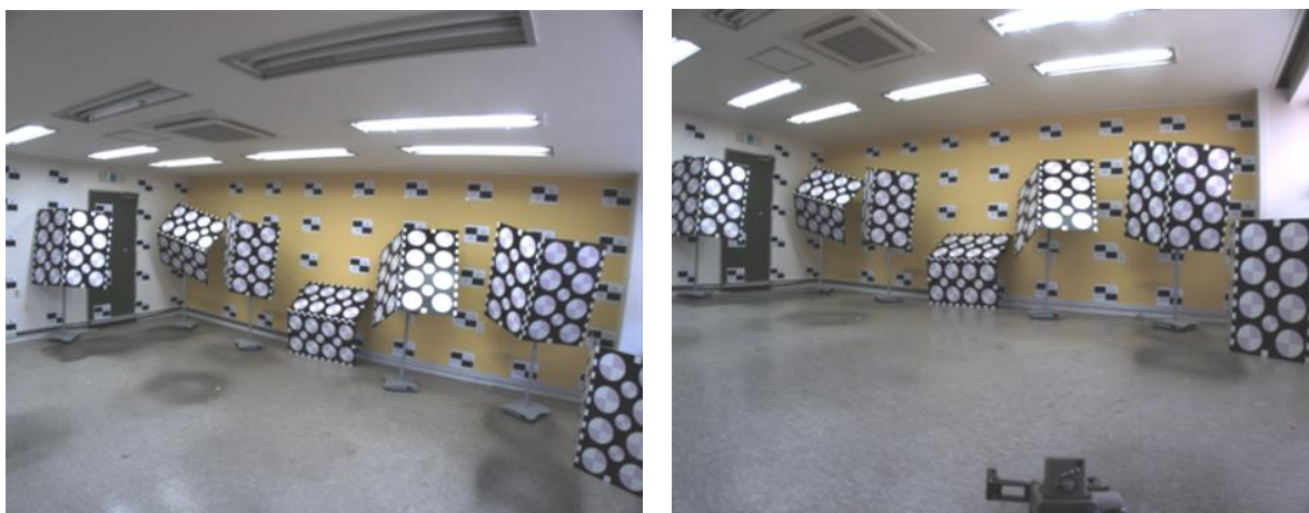
Figure 5. V-type targets setting-up for system calibration (left: 150cm height, right: 65cm height)
