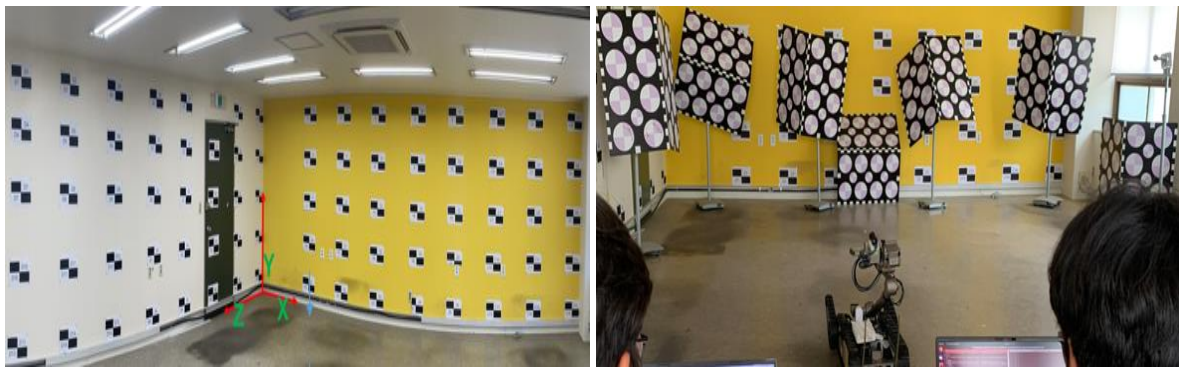
Figure 3. Calibration test-bed of investigation robot (left: camera calibration, right: system calibration)
