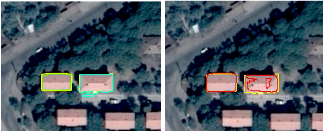
Figure 4: The RGNIR band combination left is beloveld to MRS, and the right is beloveld to SAM in Region I. (The yellow line is Ground Truth, the Green is MRS, and the Red line is SAM).
