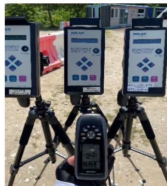
Figure 1: location of sites (left) and measurements using MICROTOPS II sun photometers(right).
