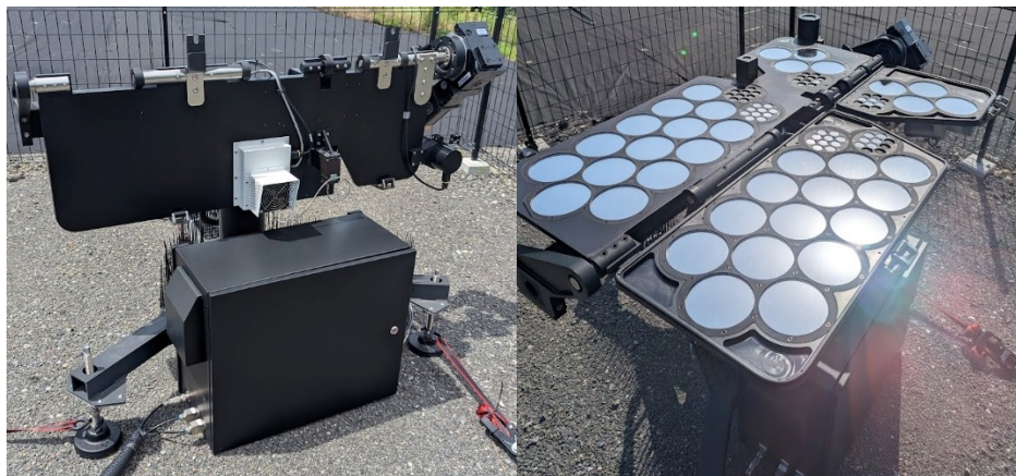
Figure 1: The automated mirror array turret assembly when closed (left) and open (right).
