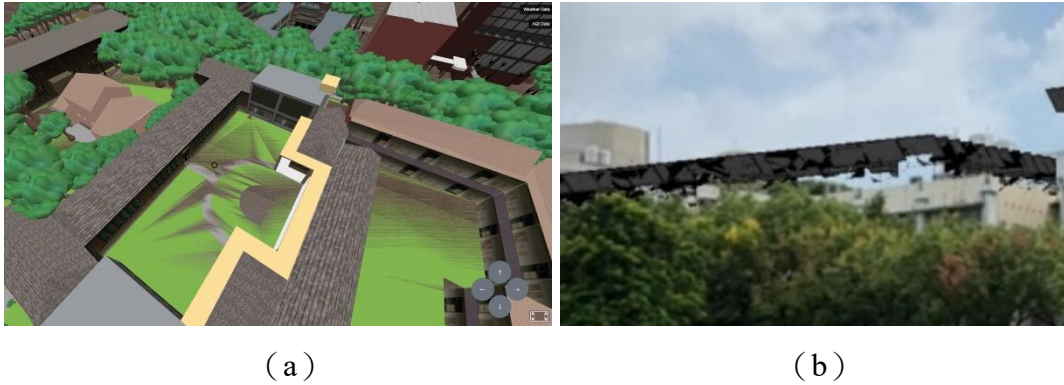
Figure 17: The z-fighting phenomenon in (a) VR and (b) AR.
