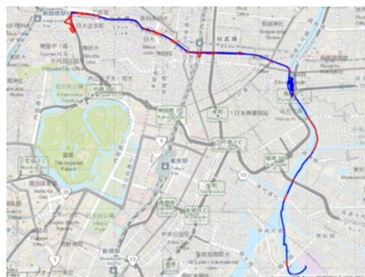
Figure 6: CLAS Positioning Mapping Result (the Kanda River).
