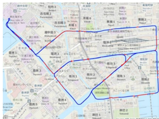
Figure 5: CLAS Positioning Mapping Result (the Shiomi Canal).
