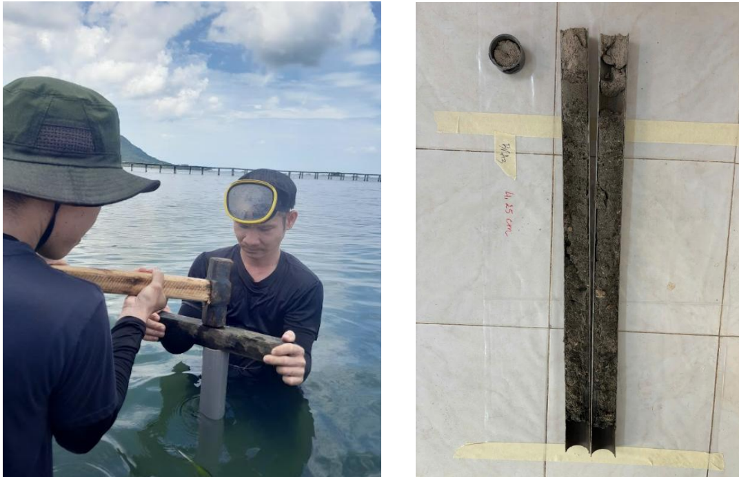
Figure 1 Preparing and inserting PVC corer to collect sediment cores
