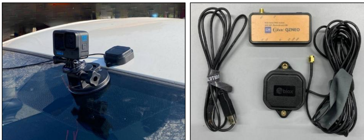
Figure 3: (Left) GoPro12 and GNSS mounted on the car. (Right) U-Blox ANN-MB-00 and QZNEO
