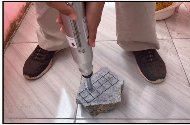
Figure 5 Rock sample testing process using Schmidt Hammer test equipment
