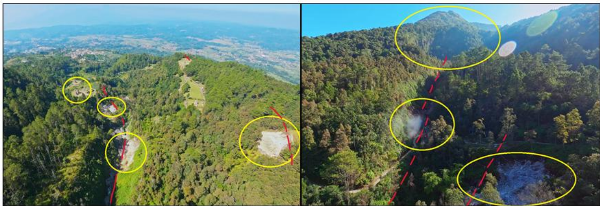
Figure 6: Drone image of fault indications in Kali Item with a strike/dip fault plane of N200°E/50°, associated with alteration zone and up flow manifestations.
