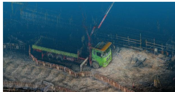
Figure 14 : Coloursied LiDAR Point Cloud to Check Adequacy of Safety Measures
