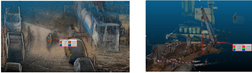
Figure 15 : Coloursied LiDAR Point Cloud to Identify Danger Zones
