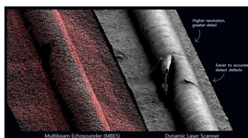
Figure 6 : Comparison of Resolutions Between Underwater LiDAR and Multibeam Echosounder
