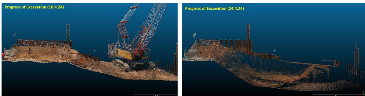
Figure 10 : Colourised LiDAR Point Cloud to Check Construction Sequence
