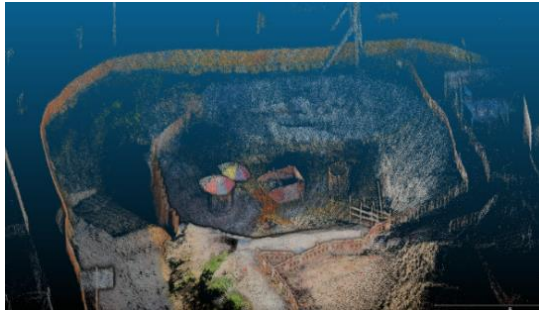
Figure 11 : Coloursied LiDAR Point Cloud to Measure Dimensions of Excavation
