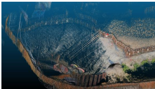
Figure 14 : Coloursied LiDAR Point Cloud to Check Adequacy of Safety Measures
