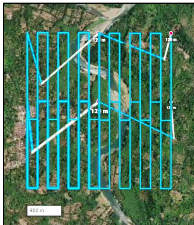
Figure 3. Aerial mapping's flight plan of the proposed site of Walimpong Dam (Modified from Dronelink, retrieved in 2025)
