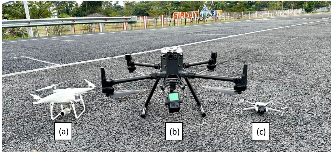
Figure 2. UAV used in this study; (a) DJI Phantom 4 Pro, (b) DJI Matrice 300 RTK, (c) DJI Mini 3
